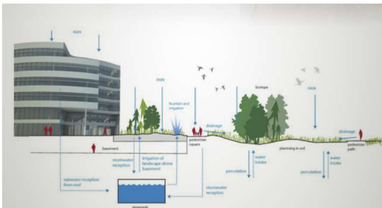
Figure 12 – Rainwater as a Resource, Water Balance Park, source (Technical University Denmark)
