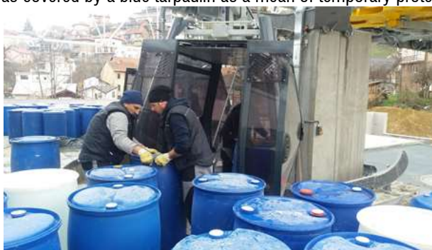
Figure 23: Placement of the test load into cabins
