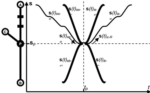
Figure 2: Classic interchange-spider with arriving (index: e) and departing (index: i) trains from/to station A (index: a), station B (index: b) or station C (index: c) as type InterCity (index: IC) or regional (index: R)
